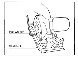
To install the blade, follow the removal procedure in reverse BE SURE TO TIGHTEN THE BOLT SECURELY.
